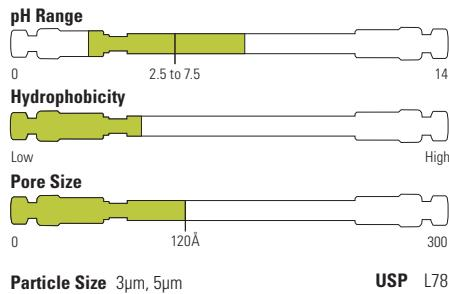
The Acclaim Mixed-Mode WAX-1 is a novel, high-efficiency silica HPLC column that combines hydrophobic and weak anion exchange characteristics. Its unique chemistry results in a multimode separation mechanism that includes reversed-phase, anion exchange, and HILIC interactions. Selectivity can be adjusted by changing ionic strength, pH or organic solvent content.
