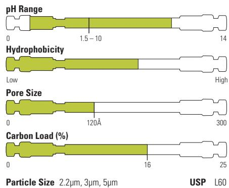
Acclaim PolarAdvantage II (PA2) columns feature a patented surface chemistry that incorporates an amide-embedded polar group and multi-point attachment between the ligands and the silica surface. This unique chemistry provides enhanced hydrolytic stability from pH 1.5-10 with 100% aqueous mobile phases and exhibits high reversed-phase capacity, with selectivity complementary to conventional C18 columns.
