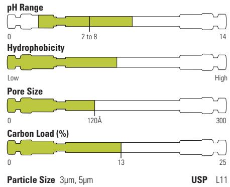
Acclaim Phenyl-1 has a higher pi-pi interaction than other phenyl phases and provides unique selectivity for aromatic compounds while maintaining sufficient hydrophobic interaction and aqueous compatibility for superior chromatographic performance.
