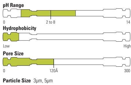
The Acclaim HILIC-10 column is designed for separating highly hydrophilic molecules by Hydrophilic Interaction Liquid Chromatography (HILIC). This column is based on high-purity spherical porous silica covalently modified with a proprietary hydrophilic layer.
