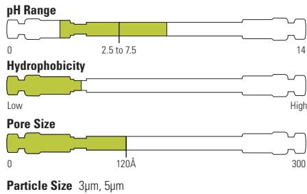
The Acclaim Mixed-Mode HILIC-1 column features a unique, high-efficiency, silica-based HPLC mixed-mode stationary phase that combines both reversed-phase (RP) and hydrophilic interaction liquid chromatography (HILIC) properties. This combination allows both hydrophobic and hydrophilic interactions to be utilized to optimize separations.
