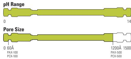
Thermo Scientific™ OmniPac™ is a range of latex-based columns. Both PAX columns have an ion exchange capacity of about 40μeq per column, and the PCX columns have a capacity of approximately 120μeq per column. The PAX-500 and PCX-500 columns separate analytes through both ion exchange and reversed-phase mechanisms, due to their higher reversed-phase capacity relative to the PAX-100 and PCX-100 columns.
