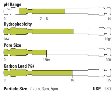
Acclaim PolarAdvantage (PA) columns feature a patented bonding column chemistry that incorporates a polar sulfonamide group with an ether linkage near the silica surface. This unique chemistry provides low silanol activity, compatibility with 100% aqueous mobile phase. The Acclaim PA column offers great separation power to resolve a wide variety of polar and non-polar analytes and supports LC-MS analysis.
