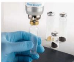
Exchangeable jaw sets for crimping or decrimping and stainless steel seals on various diameter vial
